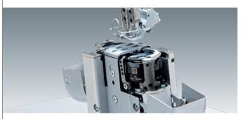
Remaining thread monitor – The photoelectric remaining thread monitor for monitoring the bobbin thread capacity is the ideal addition to class D868, especially when processing high-quality leather materials. A low supply of bobbin thread is detected early and a bobbin change is requested in good time. This prevents "sewing without thread".
