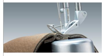
**Automatic Material Thickness Detection (MTD)** – All subclasses of the D868 e-con are equipped as standard with a device for measuring the material thickness underneath the sewing feet. With this measured value, essential sewing parameters such as thread tension, stitch length, sewing foot stroke, sewing foot pressure and sewing speed can be actively influenced during the sewing process in order to optimally adapt the sewing result to the requirements.
