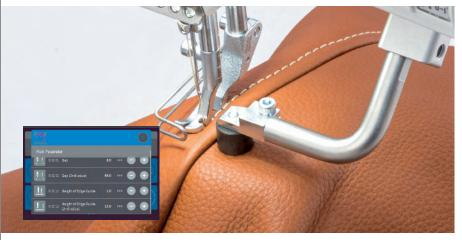
The D868-190922-01 is the ideal operating means for high-quality upholstery and leather applications. Optional, motor-driven and programmable edge guides increase process reliability and flexibility.
