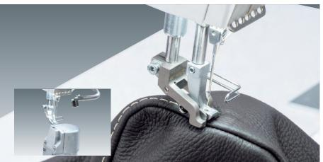
Particularly narrow radii in home upholstery applications or leather goods place high demands on the equipment. The special lap-seam foot with small area of contact and integrated edge guide enable optimum sewing results even under difficult conditions.
